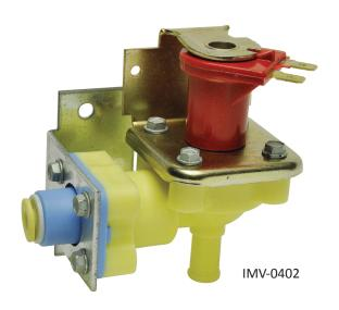
The Robertshaw® S-53 Water Valve Series is a single solenoid valve for dishwashing machines and commercial icemakers. The S-53 features the design combination of a brass inlet fitting or a quick connect fitting and a mounting bracket, which allows direct connection to the supply plumbing without applying torque to the valve body.
