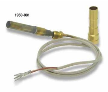
Robertshaw<sup>®</sup> thermopiles are the industry leader for gas appliance applications. Their primary function is to ensure a standing pilot light is operative so that on a call for heat, the main burner gas will be properly ignited. Thermopiles are placed in gas applications to detect the existence of a flame for safety purposes by shutting off the potential gas flow to a burner.
